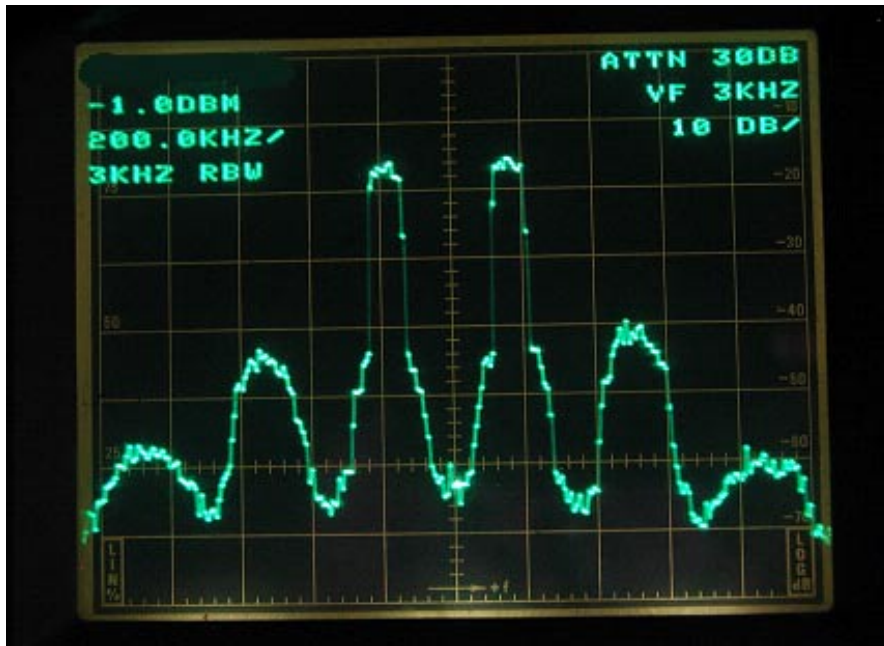
Figure 6 Sample from Digital Transmitter at full TPO prior to High Power Combining
